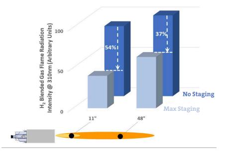
and without oxygen staging. The radiation intensity corresponding to the OH peak at 310nm, as shown on the y-axis, shows greater intensity in the 11" and 48" locations for the case with no oxygen staging (i.e.,  $H_2$  flame is shorter). When oxygen staging
