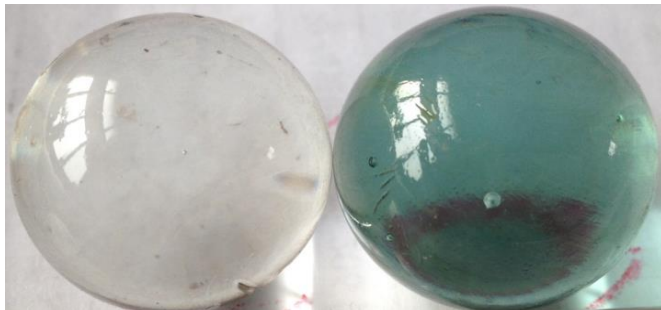
Figure 6. Photo of glass product produced with syngas firing (left) and petcoke firing having high vanadium content and poor combustion (right).
