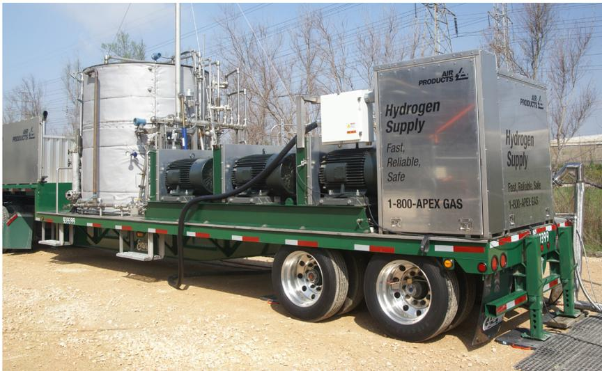
Our proprietary mobile Cryogenic Hydrogen Compressor (CHC) liquid supply system uses specialized delivery trailers and is professionally commissioned on your site. Depending on your requirements, our advanced system can provide a cost-effective, reliable supply mode to keep your operation online and productive.
