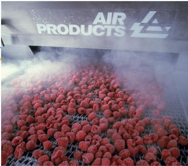
The Freshline RH immersion freezer allows you to produce consistently high-quality IQF (individually quick frozen) products, such as seafood (shrimp, shellfish), soft fruits (strawberries, raspberries) or vegetables, which can be difficult to freeze without clumping using traditional freezing methods. Instantaneous immersion freezing of the food's outer surface using liquid nitrogen helps maintain the product's form, taste and texture and prevents moisture and quality losses.
