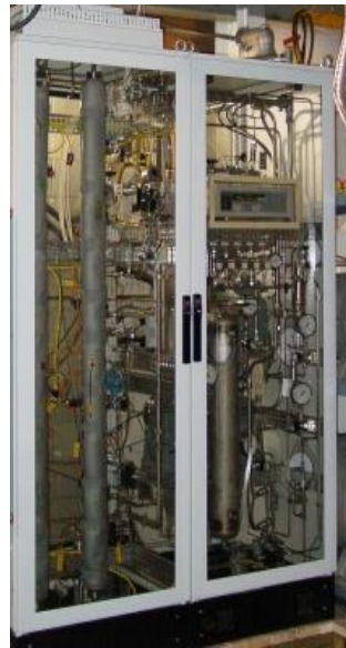
Lab scale Gasifier / PSA
