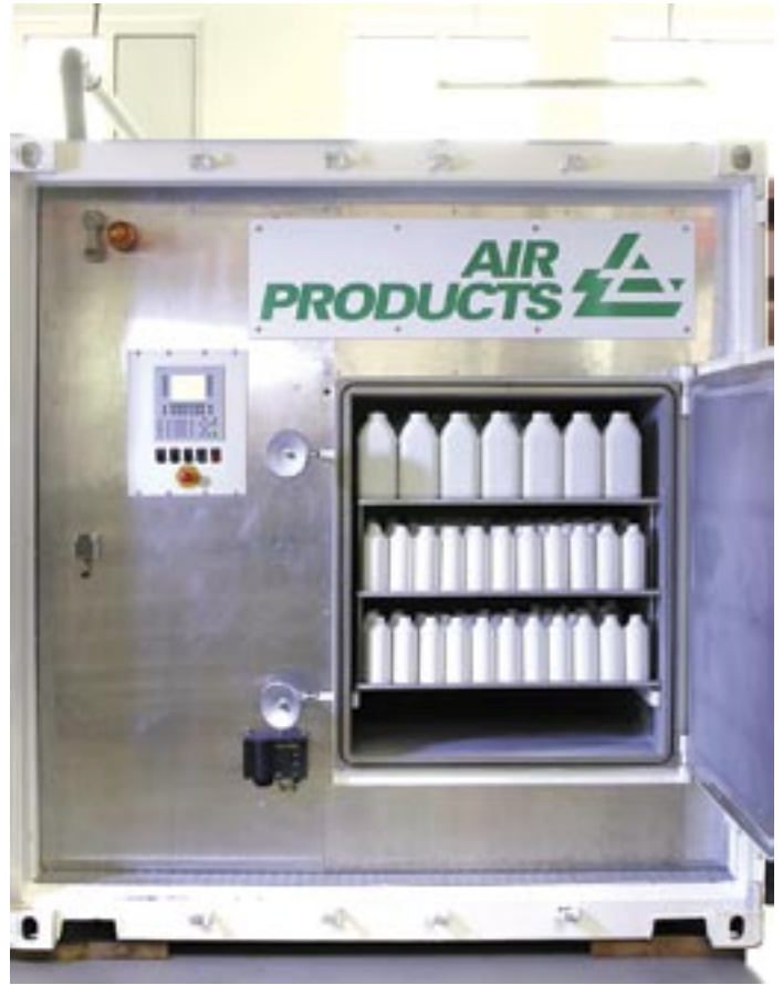
1.5m 3 "off-line" fluorination plant
